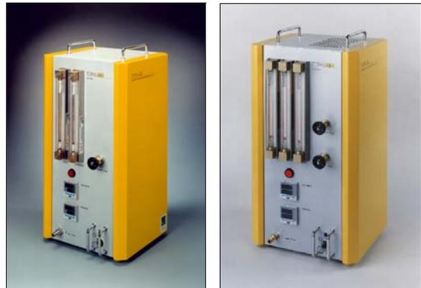
SLG250 and SLG270 Featuring the Screen Bypass Section for Larger Particles (To be seen at the Additional Flowmeter and Second Valve for Screen Bypass Adjustment)
