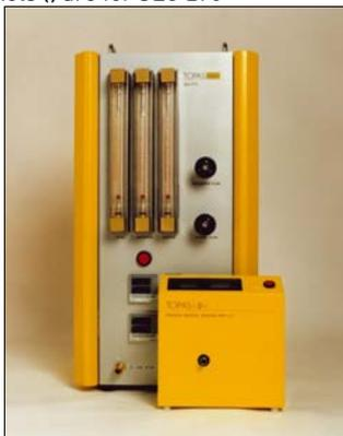
Online Monitoring of Particle Size and Concentration the Monodisperse Aerosol with the Process Aerosol Monitor PAM 510 Directly Connected to the Outlet of a SLG 270
