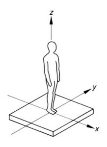
The standard defines the coordinate systems for the measurement of acceleration; x, y and z axes are always directed in the same direction but with different origins, depending on the position of the operator is sitting, standing or lying down. In whole body vibrations the z axis, which is directed in the spinal column direction, is the higher risk organ to vibrations exposure.
