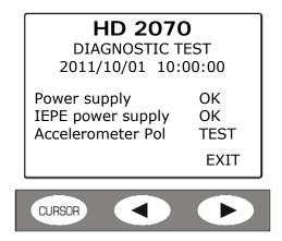
At the end it is displayed the test report; if at least one of the steps failed, the message "diagnostic error!" appears. The passed steps are marked with OK, the failed steps are marked with NO.
