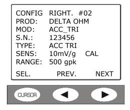
• Press **SEL** to confirm, **PREV** or **NEXT** to scroll the list of the sensors that are in the memory.
