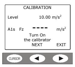
Switch on the calibrator and press FORWARD.
