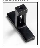
The HD2030AC4 is an adapter to be held between the hand and the handle. The accelerometer is placed in central position between the middle finger and the ring finger or between the index and the middle fingers. Light alloy made, it is suitable for anatomical shape, non-cylindrical and/or small dimension handles.
