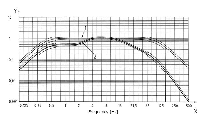
Weighting filter Wm Filter for building transmitted acceleration on persons (all directions) (ISO 2631-2)
