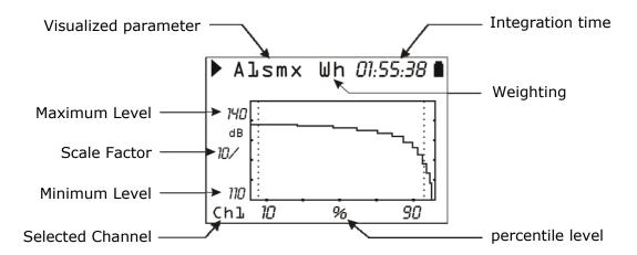
Percentile screen presents in graphic form the percentile levels from  $L_1$  to  $L_{99}$  associated with the parameter visualized in the PROFILE screen for each of the 3 channels.
