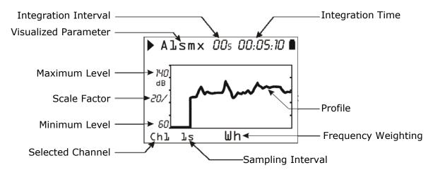
This screen presents in graphic form the profile of a frequency weighted parameter related to each of the 3 measurement channels.
