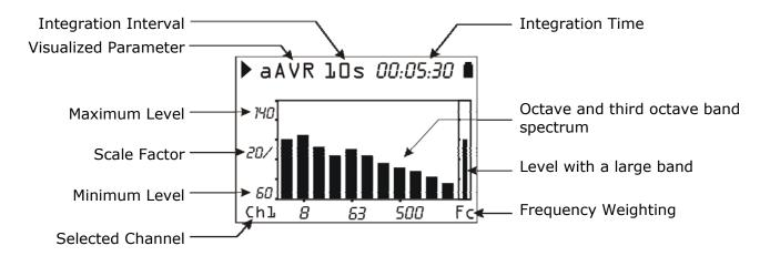
The SPECTRUM screen presents in graphic form the octave or third-octave bands spectrum related to each of the 3 measurement channels. The order of the visualized spectrum, in octave or third-octave bands, is set entering the Menu >> Parameters >> Spectrum Analyzer >> Order.
