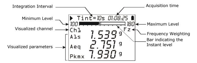
The VLM screens shows, in numerical form, three frequency weighted parameters related to each of the three measurement channels or to the acceleration vector calculated with the data of the first three axes. It is possible to scroll in sequence the screens using the right and left cursor keys.
