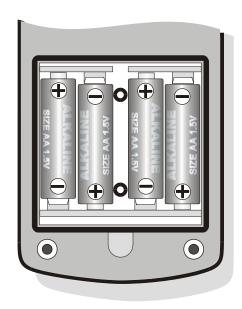
Instead of alkaline batteries, it is possible to use rechargeable batteries NiMH type.
