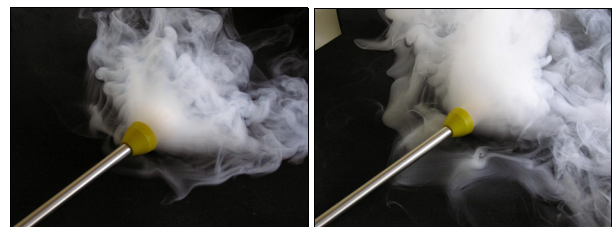
Fog output from an injection probe of the CFG 290
