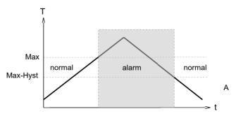
switchover delay time  $(t_{DS})$  can be applied to the switchover to the alarm state. Equally, one switch-back delay time  $(t_{DR})$  of several can be applied to switching back to the normal state.
