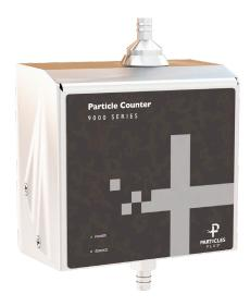
The Particles Plus® 9301 and 9501 Remote Airborne Particle Counters are designed for continuous monitoring in cleanrooms and other controlled environments. With 30 user-selectable particle size channels ranging from 0.3 or 0.5 up to 25.0 µm and a flow rate of 0.1 CFM (2.83 LPM), these instruments deliver targeted contamination detection with real-time data collection and configurable alarms for immediate incident reporting and local visual alerts.
