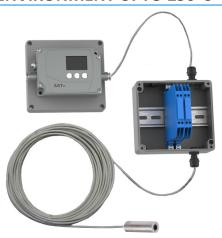
EL50-H+ Ex is a digital Pyrometer in economic range with extended sensor head in 4 wire technology, for non-contact temperature measurement between 0°C to 800°C.The sensor head is unaffected by electromagnetic interferences. The pyrometer sensor head is specially designed to withstand ambient temperature upto 250°C without cooling.
