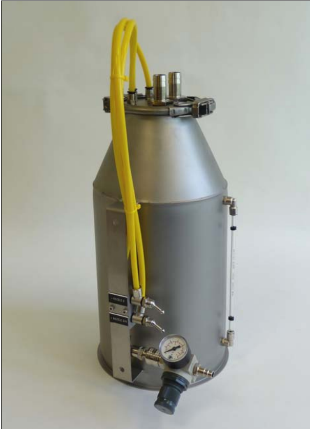
ATM 241 Aerosol Generator
