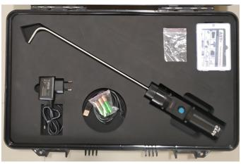
The P-GM+ (Portable Glass Mould Pyrometer) is a hand held, battery powered Non-Contact pyrometer designed primarily for the measurement of mould temperatures in container glass industry. It gives an instantaneous reading of the temperature and data logging with the press of a single switch.
