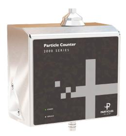
The Particles Plus® 2301 and 2501 Remote Airborne Particle Counters are designed for continuous monitoring in cleanrooms and other controlled environments. With four particle size channels ranging from 0.3 or 0.5 up to 25.0  $\mu$ m, these instruments deliver targeted contamination detection with real-time data collection and configurable alarms for immediate incident reporting and local visual alerts.
