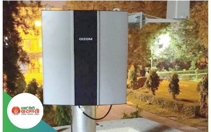
Varanasi Municipal Corporation had to monitor the increasing pollution in the city mainly due to increased tourism and infrastructure developments. Oizom deployed its Polludrone™ in the city to analyze the pollution and meteorological parameters. The solution helped in devising a graded action plan to combat pollution.
