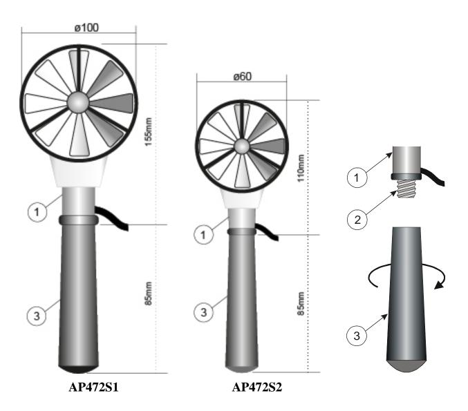
To mount the telescopic rod on the probes, unscrew the handle (3) holding the probe body still in the point (1). Screw the rod end on the screw (2). The handle (3) is screwed on the telescopic rod.
