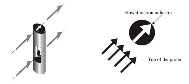
The probe should be maintained orthogonal to the flow and not tilted in relation to it:
