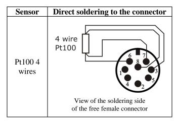
**4-wire Pt100 sensors** can be soldered directly to the pins of the free female connector without making use of the TP47 board. The 4 wires of the Pt100 sensors have to be soldered as indicated in the figure on the left.
