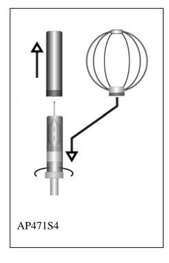
The AP471S1, S2 and S3 probes are fitted with a cylindrical protection screen that can slide longitudinally over a groove. The screen has two end-of-travel positions that block it in measurement condition (completely low) or rest condition (completely high). To reduce the space occupied when not used, the AP471S4 is supplied with a protection cylinder that can be screwed on the probe's head.
