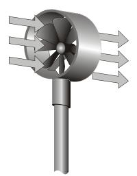
The probe should be maintained orthogonal to the flow and not tilted in relation to it
