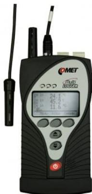
Battery powered datalogger with built-in CO2 and atmospheric pressure sensor and 4 universal inputs for measurement of temperature, humidity, 0-10V voltage, 0-20mA current, two-state signal and for counting pulses. Multilogger can be installed permanently to Ethernet network or work as portable device.
