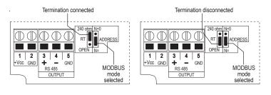
The cable shield must be connected to both line ends. The cable should have the following features:
