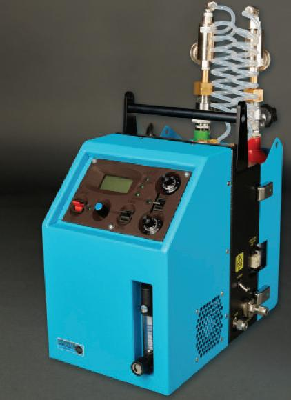
Portable Flame Ionisation Detector (FID) analysers for the discontinuous measurement of the mass concentration of gaseous and vaporous organic substances in stationary source emissions.
