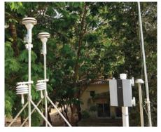
**Collocation Calibration** The sensors are calibrated against a reference station before installation and their performance is tested in the ambient condition before final deployment.
