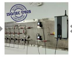
Lab Calibration Laboratory calibration is performed for Baseline Correction & Span-Calibration for all the parameters to compensate for cross-sensitivity and ensure higher data accuracy.
